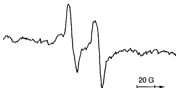
FIG. 7. ESR spectrum observed during radical polymerization of 2BCPhMI with MAIB in benzene at 60^\circ\text{C} . [\text{2BCPhMI}] = 1.0 \text{ mol/L} , [\text{MAIB}] = 2 \times 10^{-2} \text{ mol/L} .
